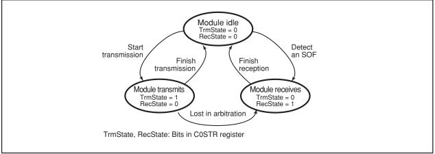
Figure 18.14 Sub Modes of CAN Operation Mode
